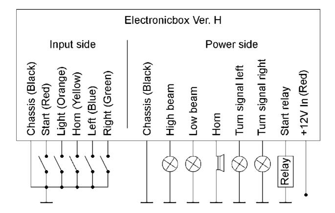
**Push button or switch input for the left flashers (blue):** You can use this input for a push button or a switch what will connect the input to ground / chassis when pressed. An close contact will start the flasher left.
